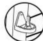
**Survey points** represented by a dot or small circle followed with a number. These were the points used for surveying. Unlike, on the surface, these markers are found on the ceiling, instead of the on the ground. Typically, they are a copper or brass metal tag with the point's number attached to a wooden plug driven into a drill hole. A survey spad which looks like a flat nail with a hook is driven into the plug to hang a plumb bob. Survey points are normally, noted only on 1"= 50' scale maps.
