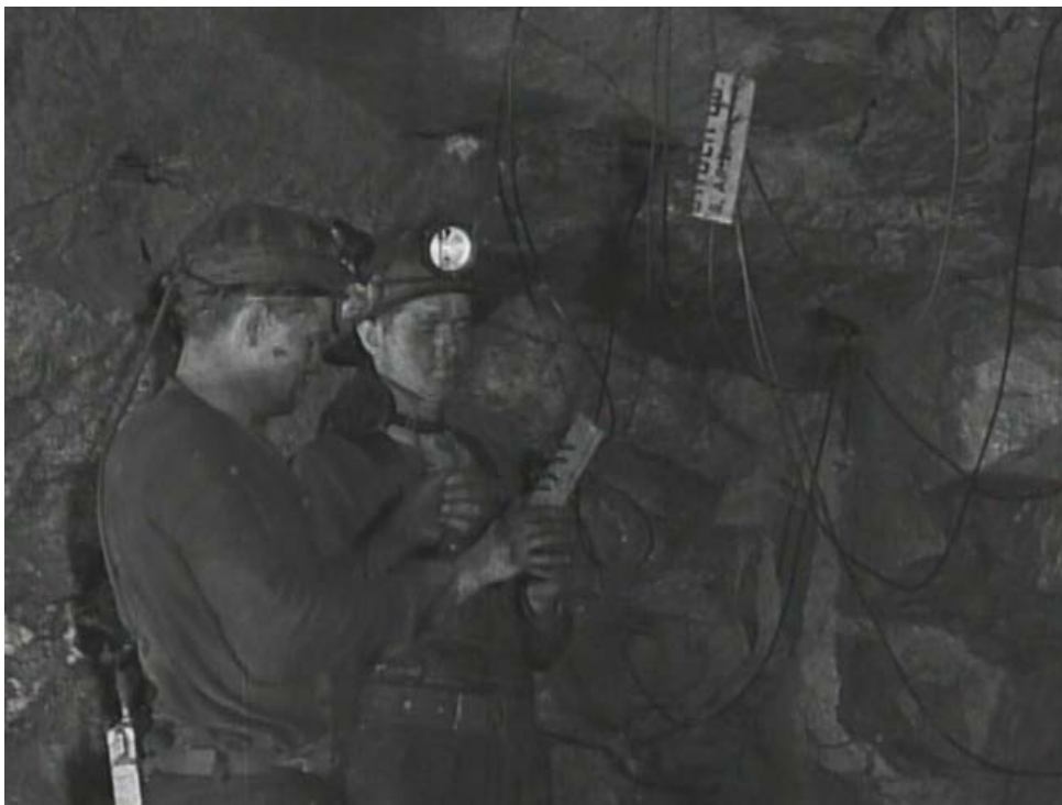
Miners in Bisbee using “Blasting Fuse Spitters” made from wooden powder boxes C. 1934
